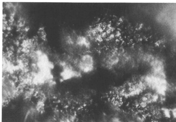
Figure 6. Optical micrograph of the residue from burning formulation of EPDM-PPO-melamine, at 300 X.
